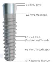
3.7 mmD Tapered SwissPlus 3.0 mmD Apex Diameter 4.8 mmD Platform with a 3.0 mmD Internal Octagon
